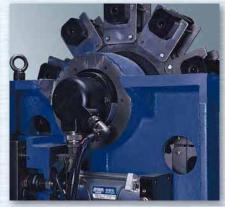
ATC magazine activated by servo motor (H500A)
